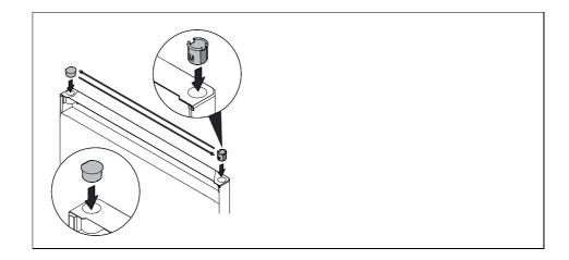
13 Insert hinge bushing and cover plug on the opposite side (the flattened sides face outwards).
