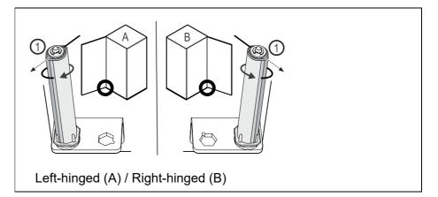
28 Turn the closing system against the resistance until the bar of the closing system (1) points outwards.
