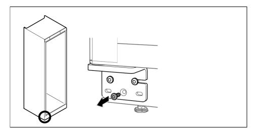
1 Remove the middle screw on the lower hinge.
