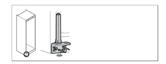
27 Screw the hinge onto the opposite side.
